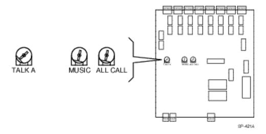
Figure 7. Communications Controller Volume Controls
